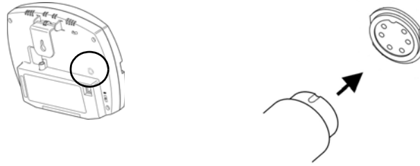
Figure 3.3: Connecting power supply to CU
